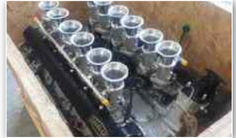
A massive 7.3-litre V12 engine awaits installation.
