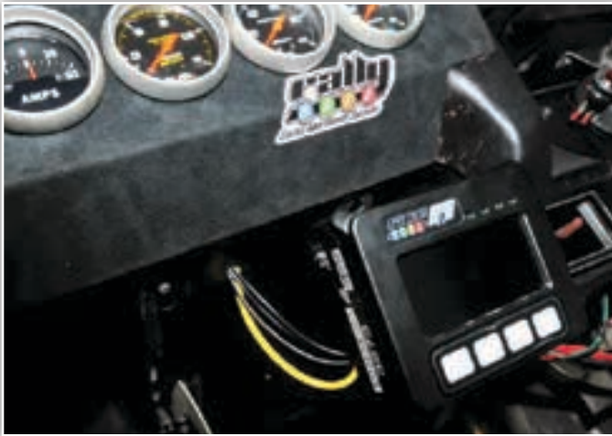
The RallySafe unit mounts to a 25mm rubber ball mount (connected through the RallySafe connector).
