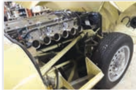
One Weber choke for each carb made balancing difficult resulting in uneven compression problems.
