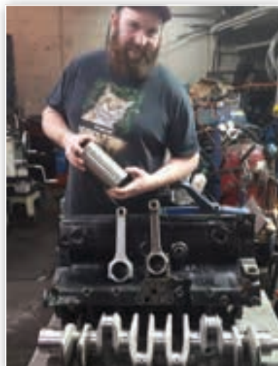
Rob Beere Racing, Coventry, supplied the 4.7 stroker XK kit -custom crank, rods, top hat liners and JE pistons plus other beautiful 'jewelry'.
