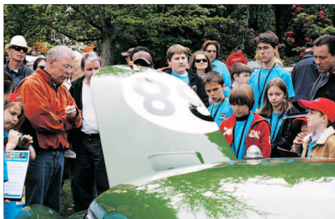
Steve Woodyard (at left, with glasses) points out one of the unique features of his 1960 MGA race car — the hood scoop is used to direct cool air not to the engine bay but to the driver's feet.
